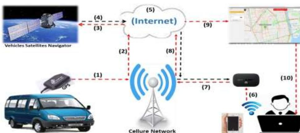
Figure No. (7): Car Tracking System Architecture
